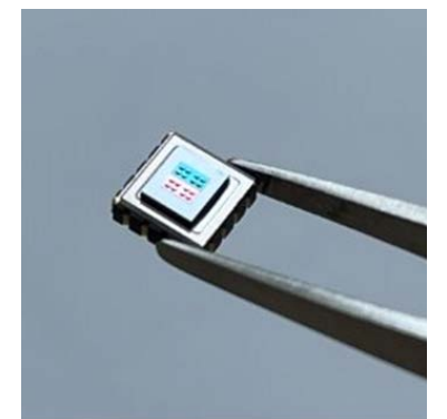
Image 45: Prototype of a CO 2 sensing module with 4 sets of 4 microlenses
