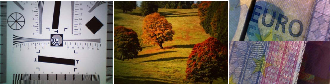
Image 49: Test images captured with an intermediate camera demo system using a 3-element f/2-objective lens suitable for automotive applications.
