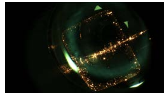
Image 56: Top view of the NIR-excited PIC Raman sensor with a droplet of analyte on top. The NIR light is propagating at the surface of the chip at the contact with the analyte.
