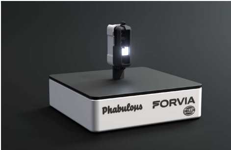
Figure 32: The final demonstrator with a vertical modular design, realized by FORVIA HELLA with the optics shown in figure 31.
