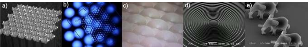
Figure 3: MLA, FMLAs, and 3D nano-structures fabricated using a) DMM, b) LMM, c) FSLA, d) GSLL and e) LMP-TPA.
