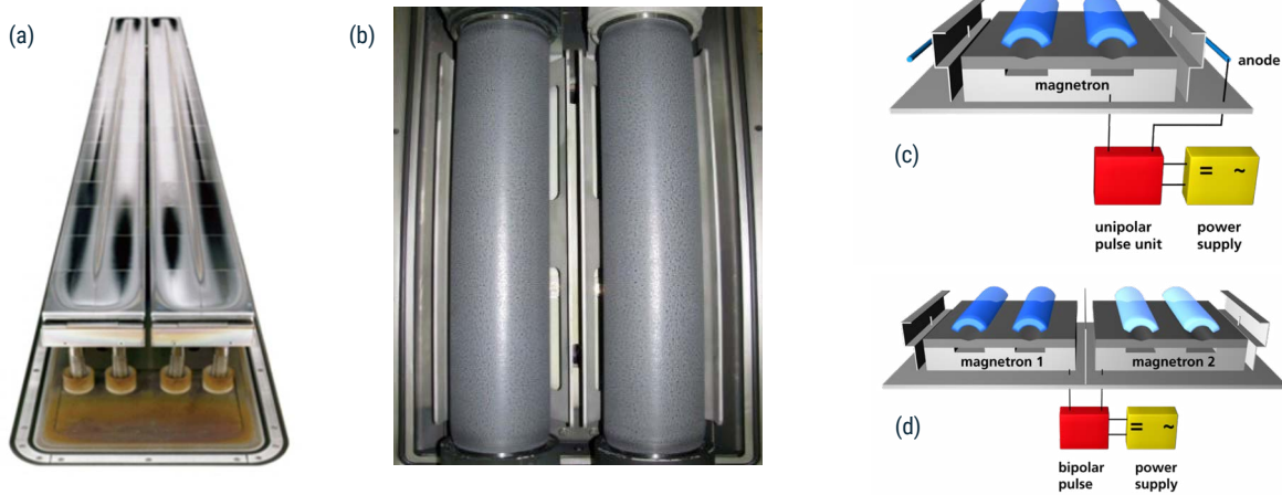
Figure 14: Planar (a) and cylindrical (b) sputtering targets. c) unipolar and (d) bipolar.
