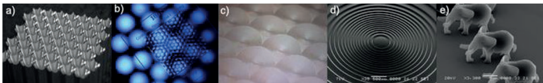
Figure 3: MLA, FMLAs, and 3D nano-structures fabricated using a) DMM, b) LMM, c) FSLA, d) GSL and e) LMP-TPA.
