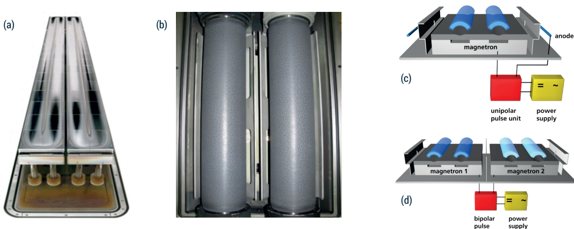
Figure 14: Planar (a) and cylindrical (b) sputtering targets. c) unipolar and (d) bipolar.
