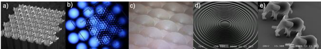
Figure 3: MLA, FMLAs, and 3D nano-structures fabricated using a) DMM, b) LMM, c) FSLA, d) GSLL and e) LMP-TPA.
