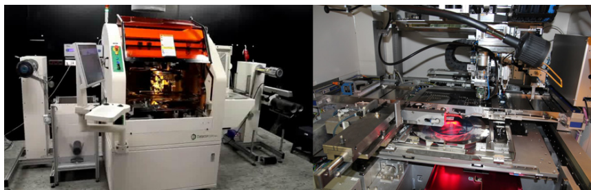
Figure 18: S2S and R2R assembly machine examples by VTT.
